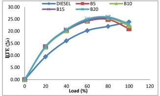
Fig.4: Variation in brake thermal efficiency with respect to change in load
