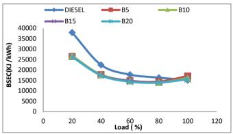
Fig. 5: Variation of brake specific energy consumption with change
