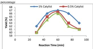
**Fig.3:** Time vs. Yield graph at 4.5:1 molar ratio for different KOH percentage.
