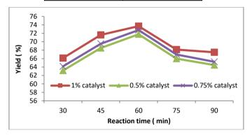
Fig. 2 Time vs. Yield graph at 6:1 molar ratio for different KOH
